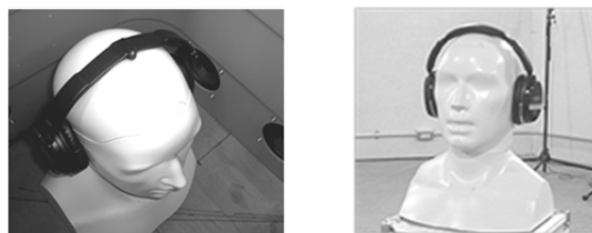
Fig. 1 NCHP measurement scenery in simulated diffused sound field (Left) Fig. 2 NCHP measurement scenery in diffused sound field field (Right)
